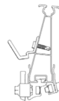
attach cable duct to rear module rail using self drilling screws, spaced two feet apart
